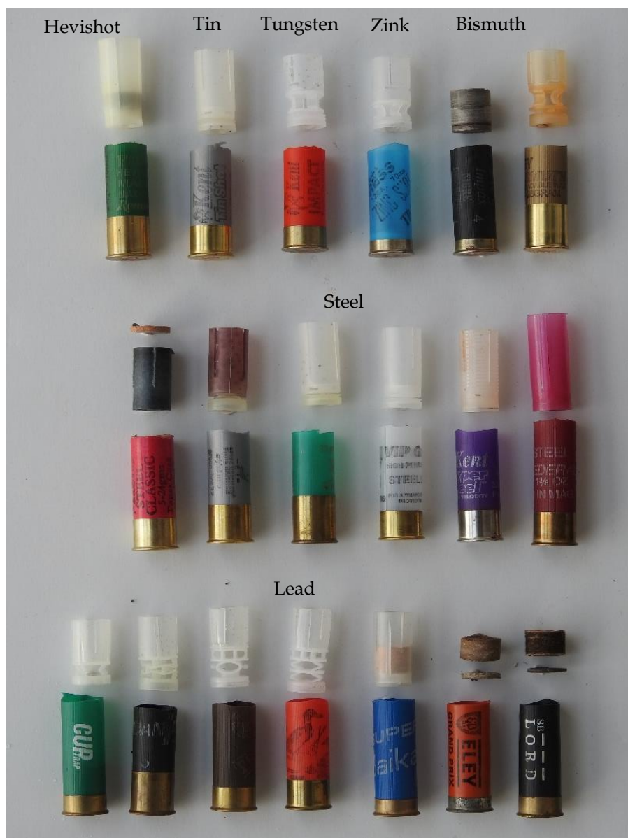
Figure 6.17. Wad construction in a selection of shotgun cartridges. All caliber 12. Bottom: lead; Middle: steel; Top (from left): he Vishot, tin, tungsten, zinc and two bismuth. See text for details.
