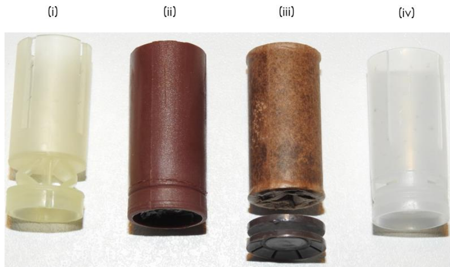
Figure 6.19. Wads made from biodegradable materials are available at the European market: (i) PVAL, (ii) PHA and (iii) fibre with a liner. Also shown is (iv) a traditional wad made from LDPE. All originate from shotgun cartridges caliber 12/70 (the most commonly used ammunition gauge).
